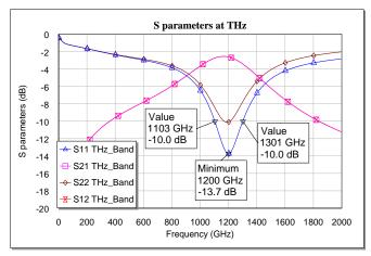
Fig. 4. Small-signal S-parameters of a planar diode (calculation)
