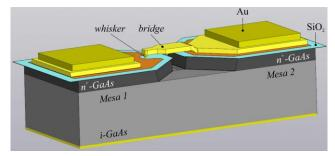
Fig. 3. The "Mesa-Mesa" structural solution of the planar Me/n- n<sup>+</sup>- GaAs Schottky diode with a whisker and an air lead (bridge) optimized for operation in the frequency range  $f_T$ =1103–1301 THz
