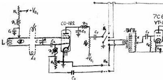
Fig. 5. Schematic diagram of Zavoisky's autodyne experimental bench.
